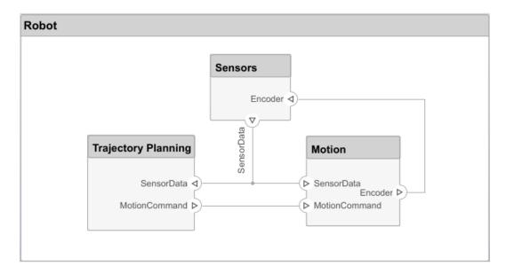
The root level of the architecture model can also have ports that describe the interaction of the system with its environment. In this example, the target position for the robot is provided by a computer external to the robot itself. Represent this relationship with an input port.
