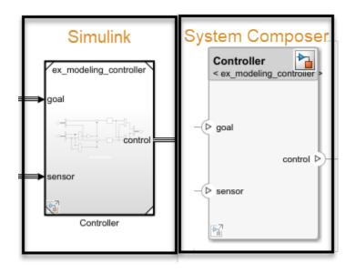
Buses at subsystem and Model block ports, as well as their dictionary links, are preserved in the architecture model.
