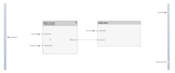
**3** Double-click **Motion Control**. Add a Sum block to subtract SensorData from TargetPosition, and add a Gain block before connecting to the output Command to represent a simple proportional controller.
