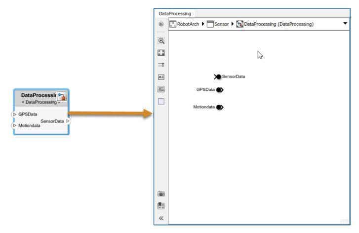
You can now go on to provide a specific algorithm implementation in the referenced Simulink model. Adding root-level ports in the Simulink model creates additional ports on the referencing component.
