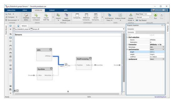
6 Complete the model using the values in this table. If a property is not in the table, you can leave it blank as it has no effect on the analysis. Pin the Property Inspector to the editor to make it permanently visible during this operation.
