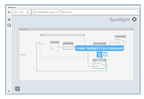
To view the architecture model at the level of a particular component, select the component and click the 📰 icon.
